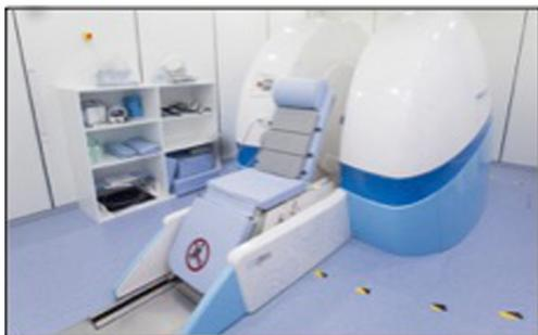
**Fig. 1** MR open 0.5-T scanner (Paramed®, Genova, Italy) with parallel magnet design
